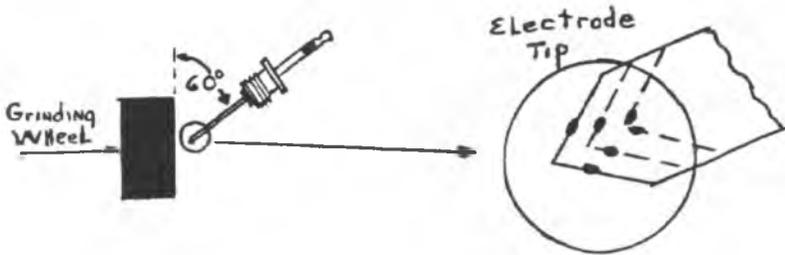
Fig. 6. Filing of Electrode Tip
