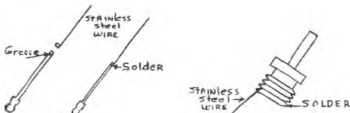
Fig. 2. Soldering of Stainless Steel Wire to Phono Jack
