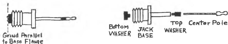
Fig. 1. Phono Jack Disassembled
